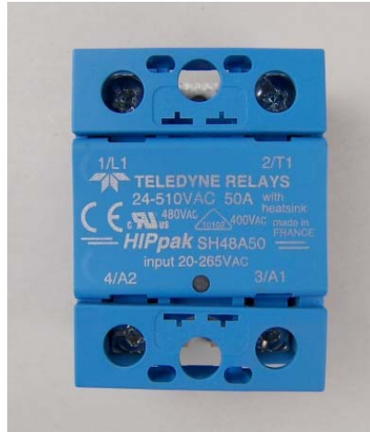
1.3751 - Solid State High Voltage Relay, 50 amps
