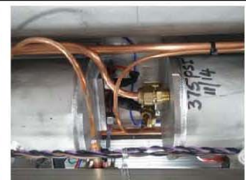
Universal brew tank with gauge tube attached
