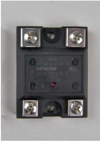
1.3740 - Solid State Low Voltage Relay, 40 amp. Used on Electrical Box Lids to Switch the Brew and Steam Elements.
