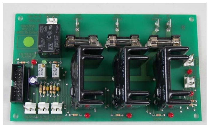
1.2163—Power Board, 3 Group Machines, Low Voltage Lid Mounted Relays for Steam Element
