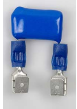
4.2780 - Snubber Assembly. Attached to 1.2133 Deltrol Pump Relay in the electrical box to reduce electrical noise spikes. 1 Per Relay.
